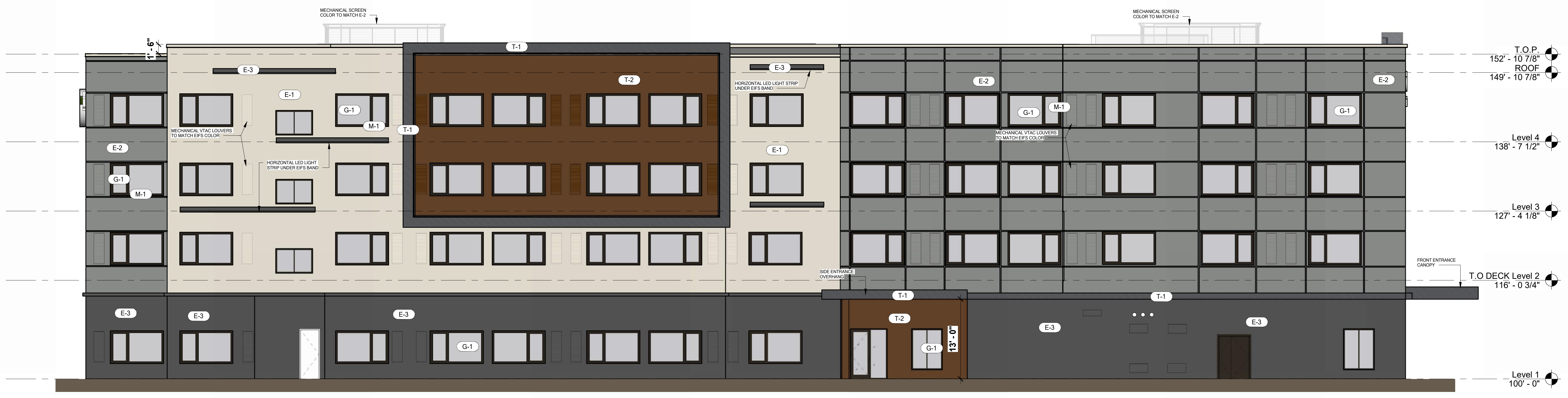
1 SOUTH BUILDING ELEVATION A019E 1/8" = 1'-0"
